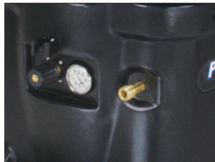
Front mounted pressure gauge on 200 - 400 p.s.i. models and recessed brass connector.
