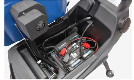
**EASY ACCESS TO MOTOR, BATTERIES AND TANKS**
