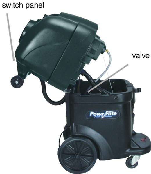
**NOTE:** There is a valve in the upper compartment that either sends the water through the heating components, or bypasses them. The machine is preset in the “HOT” position. To clean with cold water, turn the valve to “COLD” or UP position. This should be done prior to filling the tank with water. For general cleaning, it is recommended leaving the valve in the “HOT” or down position and cleaning with hot water.
