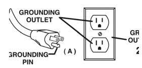
This unit is for use on a nominal 120 volt circuit and has a grounded plug that looks like the plug illustrated in (Fig. A).
