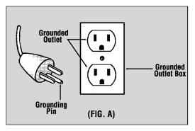
This unit is for use on a nominal 120 volt circuit and has a grounded plug that looks like the plug illustrated in (Fig. A).
