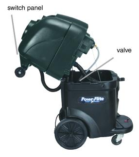
**NOTE:** There is a valve in the upper compartment that either sends the water through the heating components, or bypasses them. The machine is preset in the "HOT" position. To clean with cold water, turn the valve to "COLD" or UP position. This should be done prior to filling the tank with water. For general cleaning, it is recommended leaving the valve in the "HOT" or down position and cleaning with hot water.
