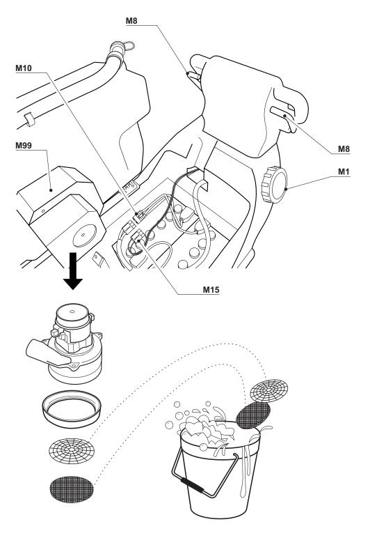
Recovery tank: weekly clean it as follows: switch off the machine, switch off the voltage, open the dirty water tank. Remove the suction motor: over M99 (page 9). Then remove the suction motor: the filter and the net will be cleaned underneath. Drain the dirty water from the M2 (page 7) pipe. Remove the dirt that has settled in the tank. To do this, open the cap M0 (page 7) to have visibility inside the tank.
