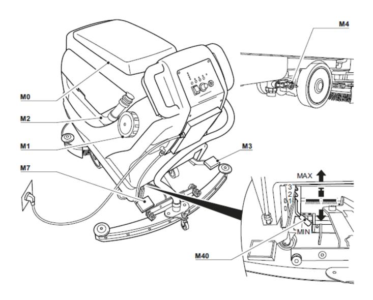
Turn the key switch to position ON (I). In this position the machine can already move backward and forward as described below. Next press butt 🖰 (control panel) then button (brush). At this point the water dosage and vacuum will start automatically. If desired, they can be switched off individuall right (wate Lind (vacuum) buttons.
