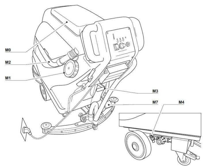
Turn the key switch to position ON (I). In this position the machine can already move backward and forward as described below. Next press butt 🖰 (control panel) then button (brush). At this point the water dosage and vacuum will start automatically. If desired, they can be switched off individuall \*with (wate \*\*Lid\*\* (vacuum) buttons.
