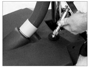
Attach the solution hose female connector to the male connector located on top of the Powr-Extractor Brush housing.
