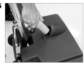
Push the vacuum hose cuff into the stainless steel manifold tube inside the middle of the Powr-Extractor Brush housing.
