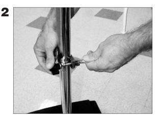
Insert hose ring bolt into clamp.
