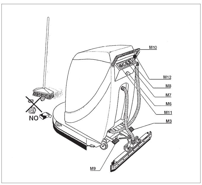
The area to be scrubbed: Debris and grit must be swept up before starting the scrubbing operation to avoid vacuum line blockage and to permit the detergent to perform efficiently.
