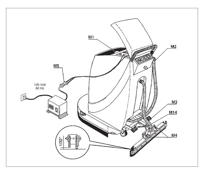
**Solution Tank:** The solution tank is located under the lid, at the front of the machine, with the filling-funnel **M1** in an accessible position for easy re-filling.
