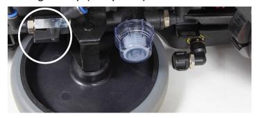
Fig 16 Solution tap fully closed
