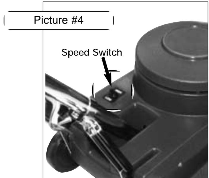
Keep the machine clean especially at the handle tube and collar so the handle tube will move freely through the collar. Inspect the cord for cuts, gashes, or loose prongs; replace as needed.
