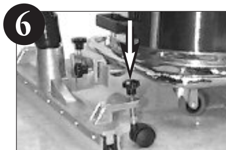
6 Adjust the height of the squeegee blades with the wheel alignment knobs on each wheel. Adjust squeegee blades to slightly contact floor surface across length of blades.
